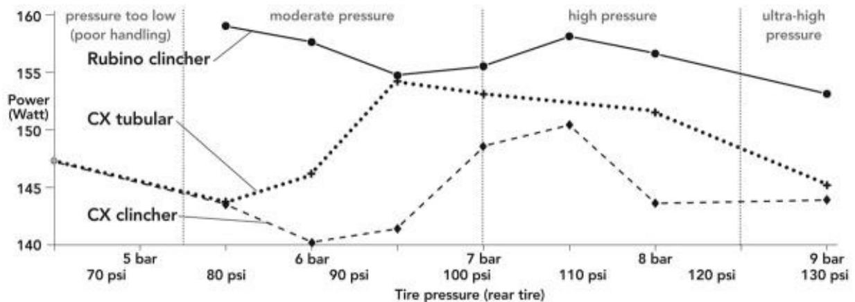
Figure 1: Performance with increasing tire pressure for three Vittoria tires.
